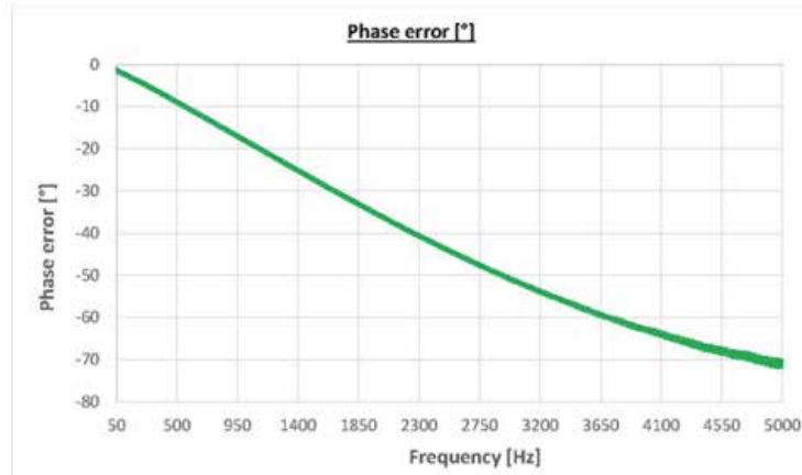
Figure 11: Frequency transmission behaviour of the RQI-3 with a FASK 150 (amplitude error and phase error)
